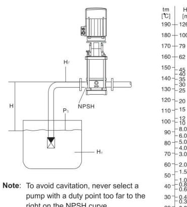
**Note:** To avoid cavitation, never select a pump with a duty point too far to the right on the NPSH curve.
