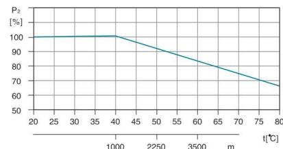
For example, when the pump is installed at altitude of more than 3500 meters above sea level, P2 will be decreased to 88%. When the ambient temperature is 70°C, P2 will be decreased to 78%.
